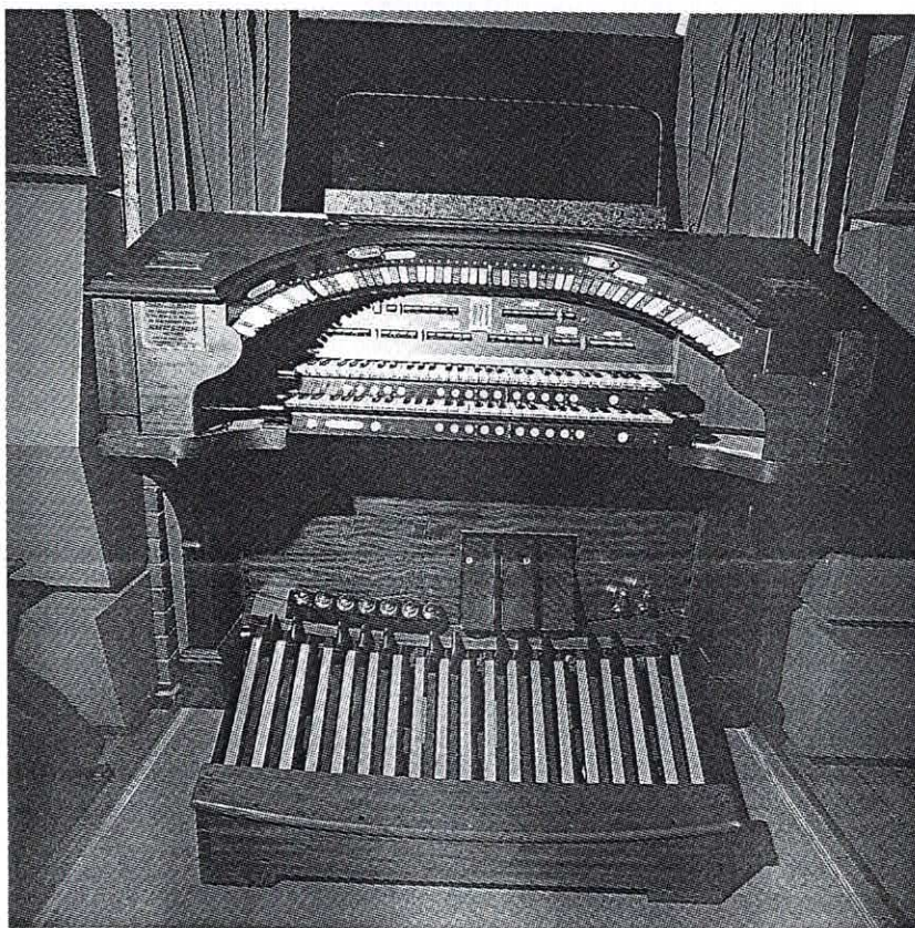
The horseshoe of the console is entirely new, having been raised 50mm to accommodate 2 tiers of stops (103 in all) on the bolster .
