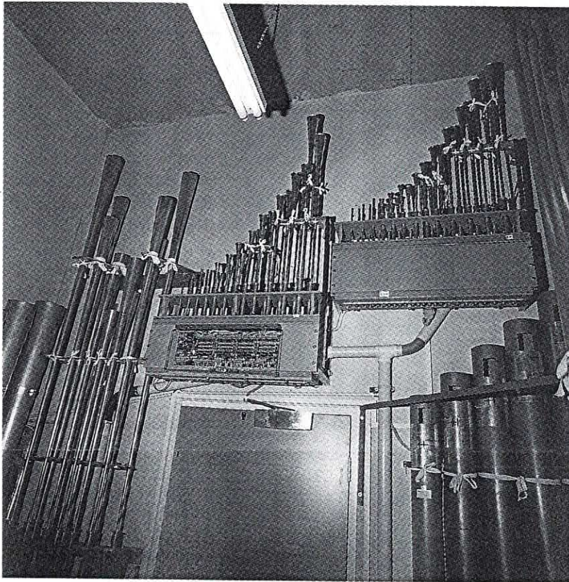
The Post Horn pipes are grouped in 3 chests. Diapason and Diaphone pipes are to the left and right respectively. Relics of a failed electronics system remain mounted on the centre chest.
