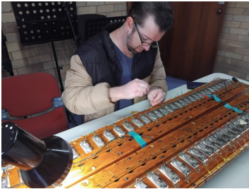
Roger Dunk soldering wires to the electromagnets
