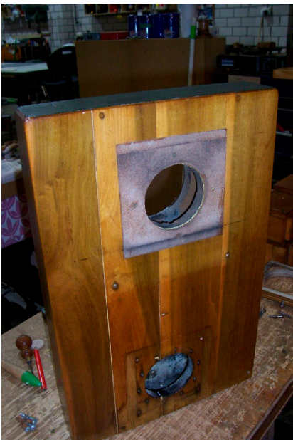
16' Tibia wind trunk restored
