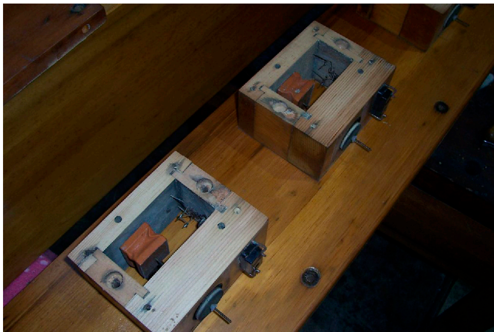
Tibia Primary blocks sanded and restored
