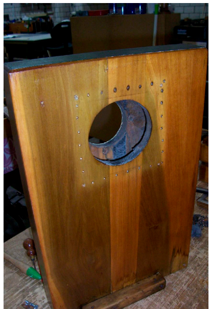
16' Tibia wind trunk restored
